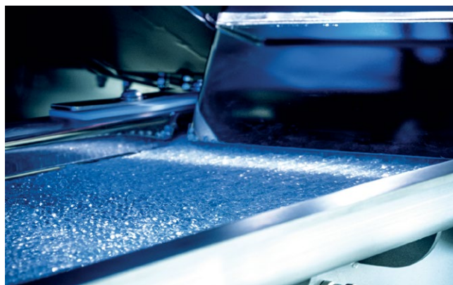
With the PURITY SCANNER ADVANCED, the pellets are conveyed to the inspection area via a stainless steel vibrating chute
