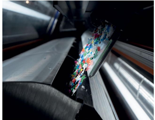
Polyolefin flake sorting
